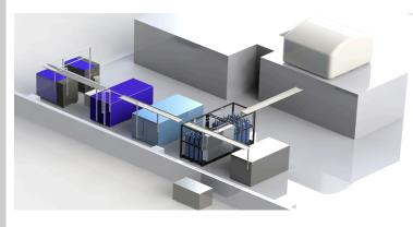
QuantumPure CS helium recovery system integrated with a VRC Metal Systems cold spray booth in MA, USA
