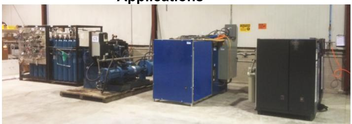
QuantumPure CS<sup>TM</sup> standard recovery and purification system for the cold spray industry:
